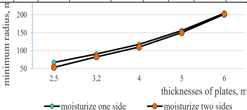
Fig. 2. Dependence of the minimum radius for different thicknesses of plates
