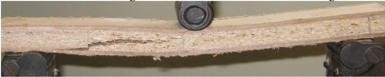
Fig. 5. Test specimen with a WPB core-board in the jacket of WFB at the moment of breakage
