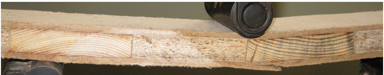
Fig. 6. Test specimen with a core-board made from RW and WPB, and in the jacket of WFB at the moment of breakage
