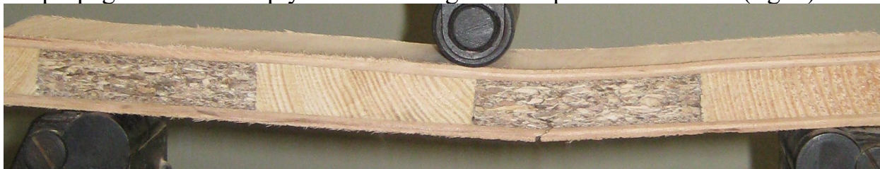
Fig. 8. Test specimen of a veneered GB with the core-board made of RW and WPB at the moment of breakage
