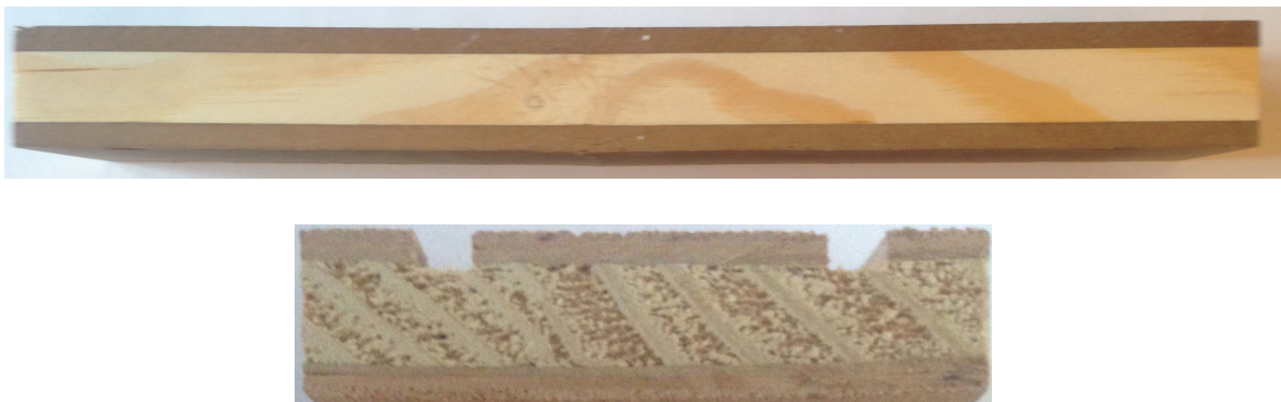
Fig. 7. Examples of front PCW-made blockboards for testing
