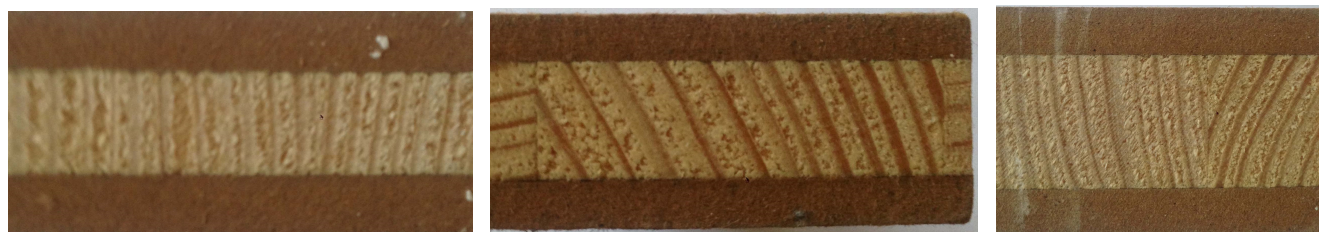
Fig. 1. Cross-section examples of front blockboards for testing
